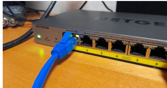
2. Connect the other side of the Ethernet cable into your network switch.
