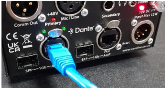
1. Plug an Ethernet cable into the primary port of the AVN-CU1.
