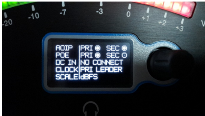
3. If your network switch supports PoE, the unit can be powered using this method and is indicated by the 'Pri' and 'Sec' icons next to 'POE' on the display.
