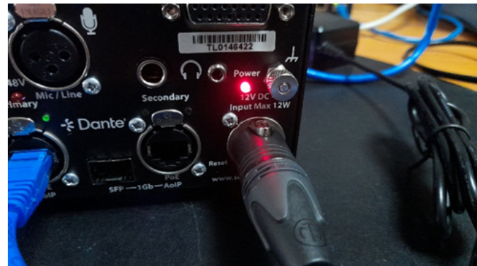
4. If your switch does not support PoE, the DC adaptor can be used instead and has the following pinout: Pin 1: Ground, Pin 2: N/C, Pin 3: N/C, Pin 4: +12V
